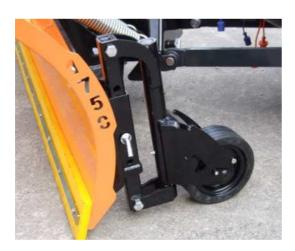
■ <u>SLEDGES</u>: they are applied to the blade by means of the specific support and they are locked with a pin and the corresponding split pin
