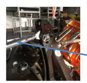
UPPER THIRD POINT OF THE TRACTOR CONNECTED TO THE SNOW BLADE
