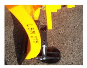
■ <u>SHOCKPROOF VALVE</u>: it is connected to the orientation cylinders to deaden eventual recoils during the work
