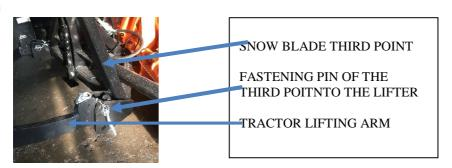
Connect the third upper point of the agricultural tractor with the mechanical screw arm to the snow blade, which is provided with a safety lock by fixing it with the specific passing pin and the corresponding safety split pin as shown in picture 3)
